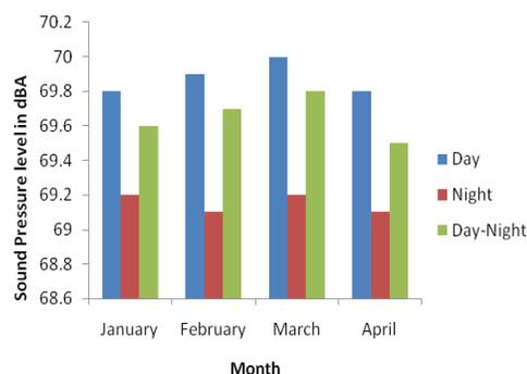
Fig. 4:  $L_{eq}$  values in dBA near South East Direction of Coal Crusher House
