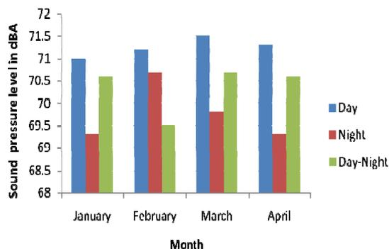
Fig. 1.  $L_{eq}$  values in dBA near Product Processing Yard
