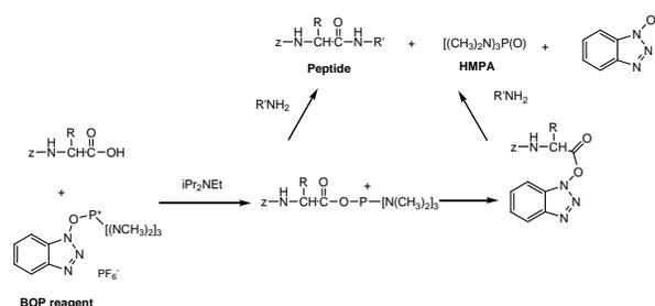
Scheme-2 Mechanism of BOP reagent
