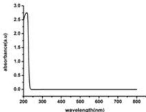
Fig.2. UV-Vis spectra of 1-butyl-3-methylimidazolium hexafluorophosphate.
