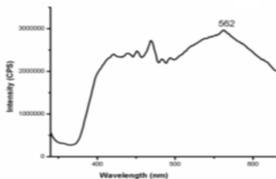
Fig.6. Photoluminescence spectra of ZnO microspheres.
