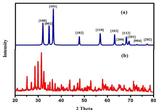
Fig.3. XRD pattern of ZnO (a) after annealing and (b) before annealing.
