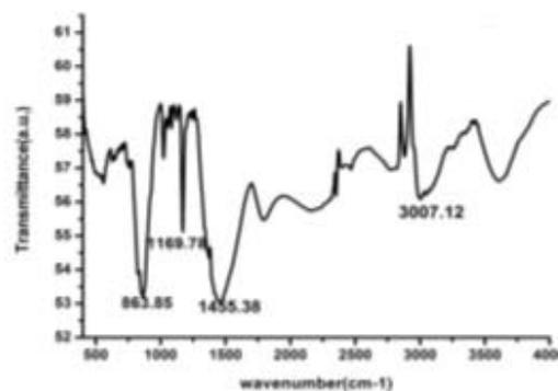
Fig.4. FTIR spectra of ZnO microspheres.
