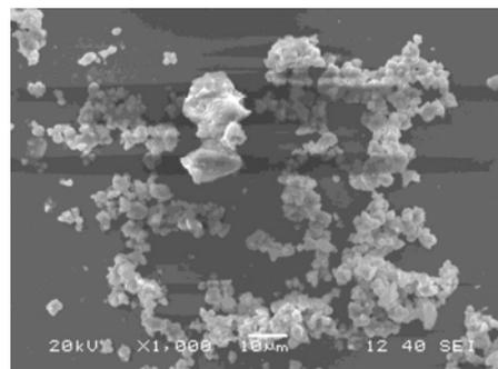
Fig.5. SEM image of ZnO microspheres.
